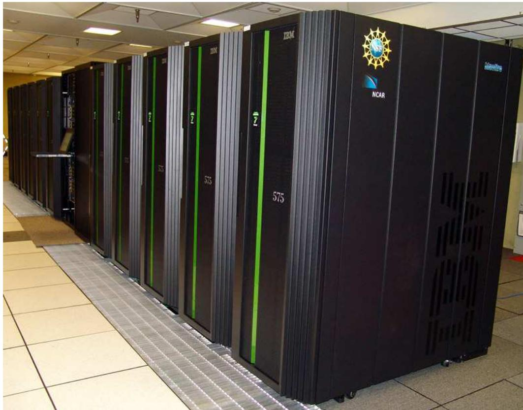
IBM Power 575: 128 nodes, 32 CPUs per node
