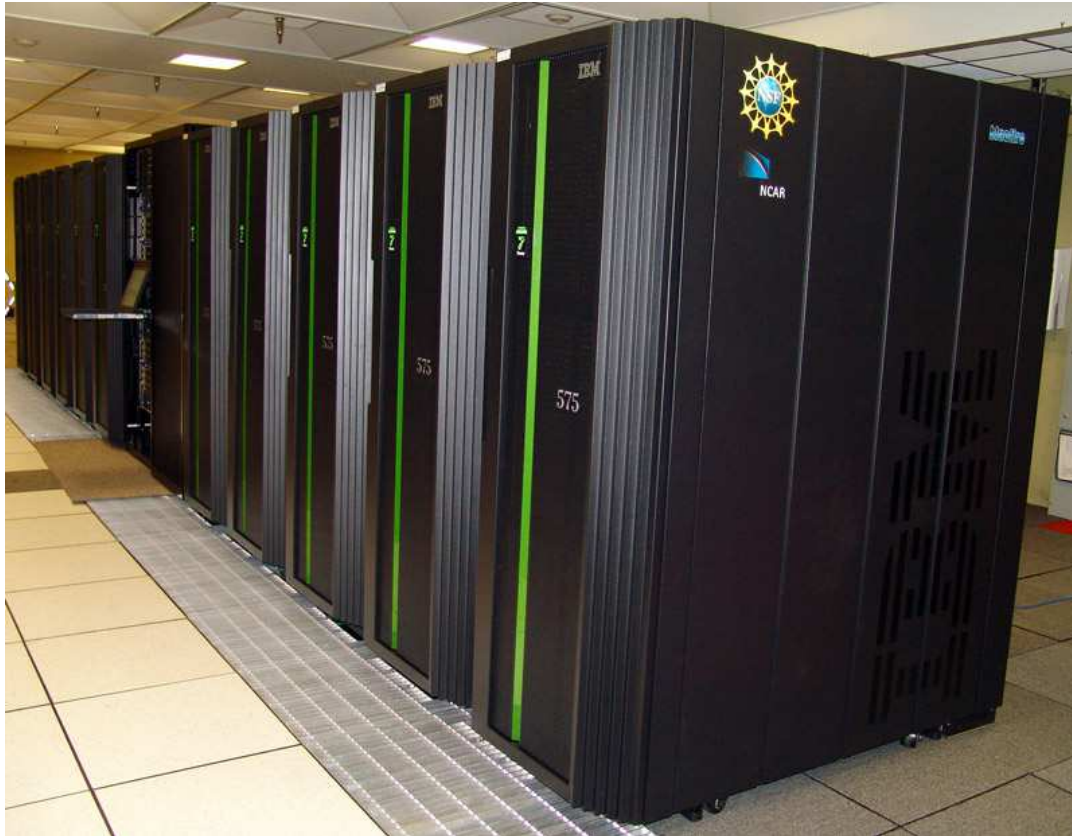
A serious cluster: NCAR's bluefire IBM Power 575: 128 nodes, 32 CPUs per node Each CPU is 4.7GHz, 4096 CPUs in total
